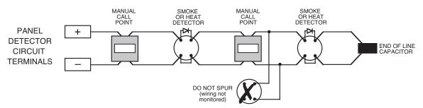
Connect an end-of-line (EOL) capacitor (provided in the panel's accessory pack) across the terminals of the last device on each circuit to allow the wiring to be monitored.
