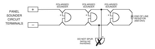
All sounders must be polarised as unpolarised sounders will show a sounder fault. A 6k8 end-of-line resistor (provided in the panel's accessory pack) must be connected at the end of each sounder circuit to allow the wiring to be monitored.
